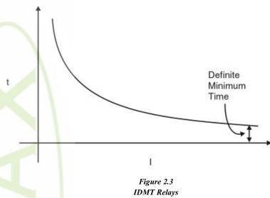
It can be seen that the operating time of an IDMT relay is inversely proportional to a function of current, i.e. it has a long operating time at low multiples of setting
