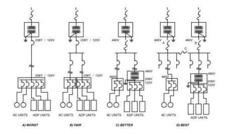
Figure 1.9 Four Wiring Diagrams
